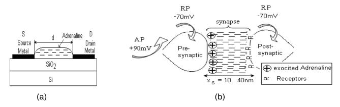
(a) A cross-section through structure; (b) The Action Potential arrival, followed by the adrenaline releasing into synapse.
